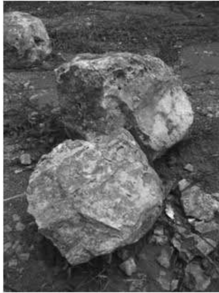
Figure 6-6: Boulders of Epithermal Quartz-Pyrite Vein Partially Oxidized
